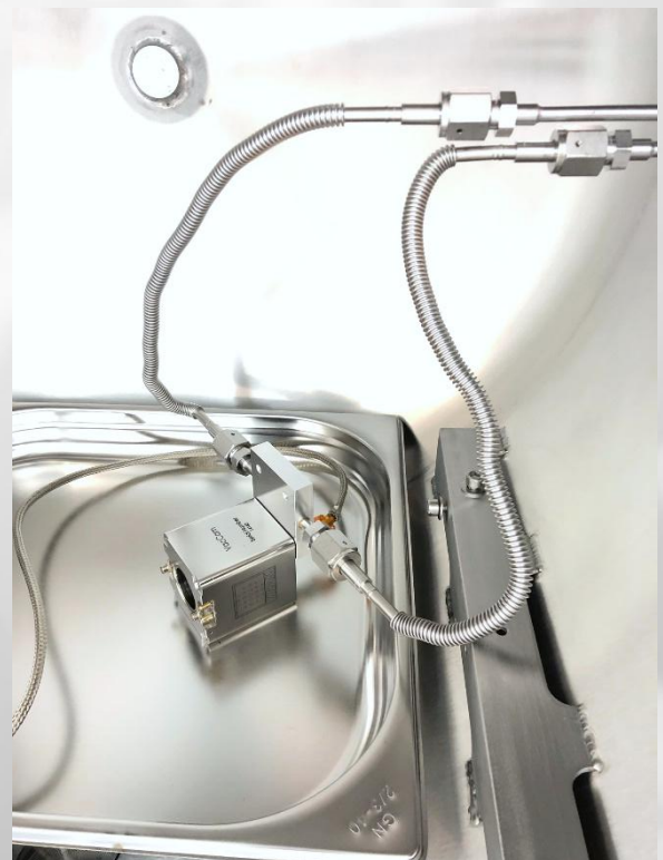
VacCam in vacuum environment with integrated thermal solution
