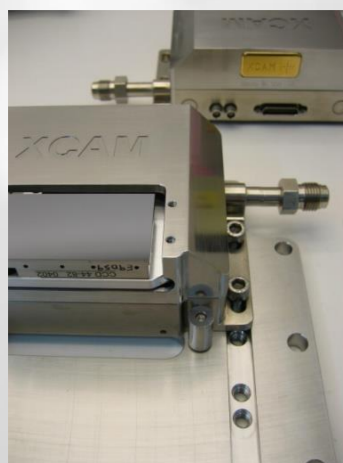
Figure 2 XCAM Single Unit on Base Plate in Foreground with Sensor Exposed to view, and (background) Alternative Orientation
