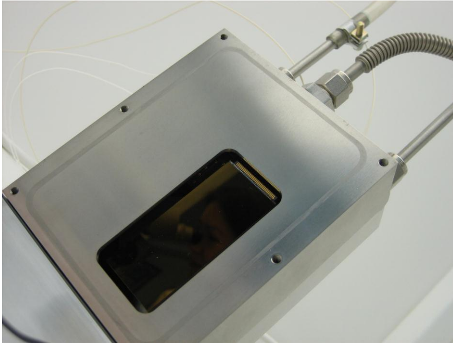
Fig 5: Alternative Format Single CCD camera, showing sensor and water and vacuum pipes
