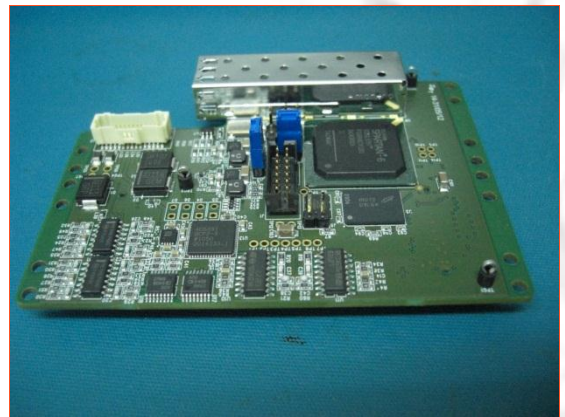
Figure 2 above the 'CHI' board (Camera Head Interface) which replaces the digital board in the stack making our vacuum cameras truly 'fibre optic'
