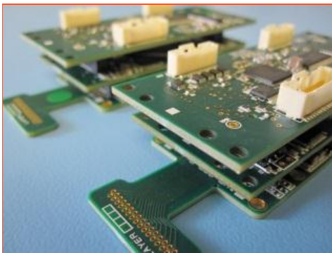
Figure 1 shows the first stage of development. One stack of 3 boards drives each detector, with each stack the width of the detector. The picture above shows two detector stacks, each one capable of driving a CCD230-42 (or other detectors with re-configuration). The boards are, from the bottom going upwards: CCD drive board, centre analogue board, left digital board.
