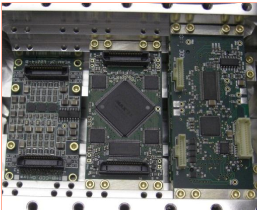
Figure 1 shows the first stage of development. One stack of 3 boards drives each detector, with each stack the width of the detector. The picture above shows two detector stacks, each one capable of driving a CCD230-42 (or other detectors with re-configuration). The boards are, from the bottom going upwards: CCD drive board, centre analogue board, left digital board.
