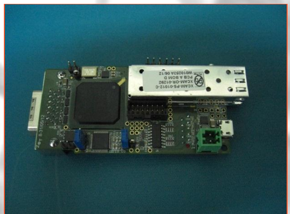
Figure 3 below – the FGA board which can be used as a fibre optic transceiver for many applications.
