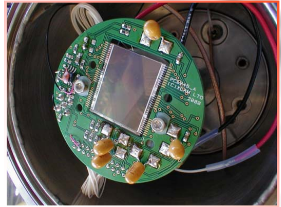
Figure 1 A prototype custom CCD and headboard developed by Xcam Ltd for this work
