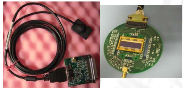
Fig 2: (Left) The CCD38 used for evaluation of high signal handling capacity CCDs, and (right) the CCD30-11 used for radiation damage studies
